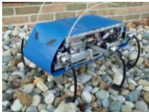
Figure 1: The RHex experimental platform.
