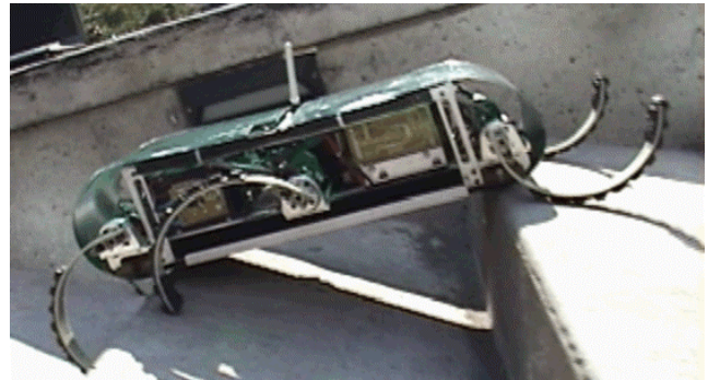
Figure 5 - Sticking on shallow stairs
